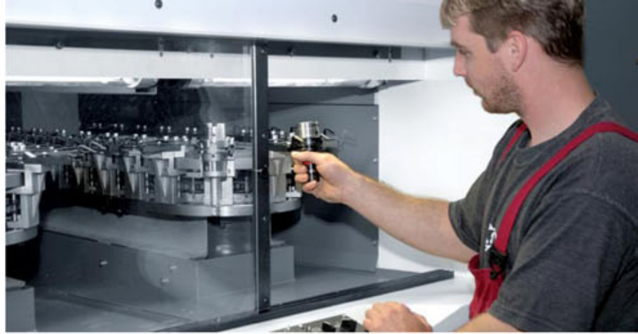
↑ Tool magazine loading in the rear part of machine
