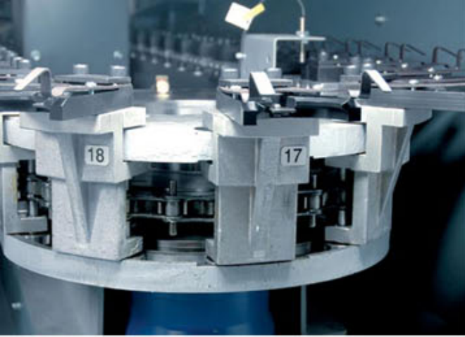
↑ Pick up tool magazine - 32 / 64 stations
