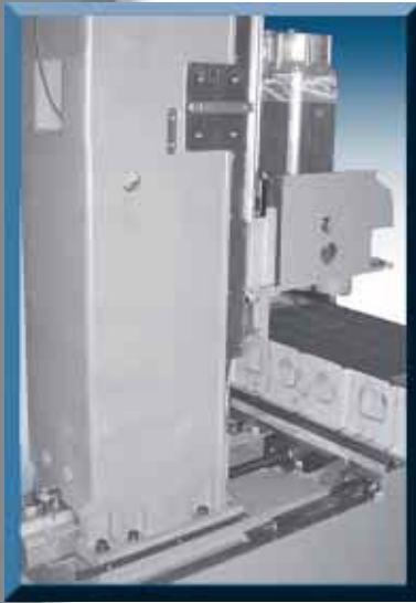
Each VMC machine begins with precision ground heavy-duty casting mated together to the highest standards.
